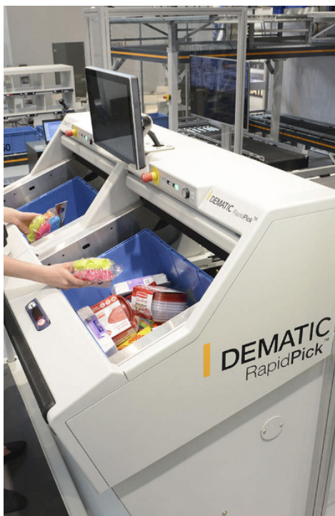
Figure 14 : exemple : station fixe RAPID PICK de DEMATIC
